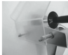
2. Attach the hand guard.
